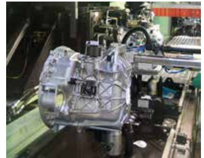
Transmission in standby position in front of clamping station
