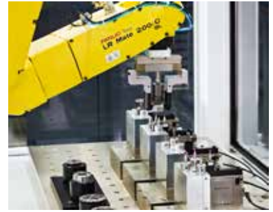
Part handling by 6-axis robot – internally as well as with adjacent machines
