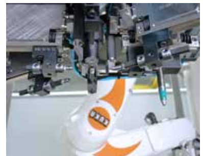
Post-process measuring cell for pump rotors
