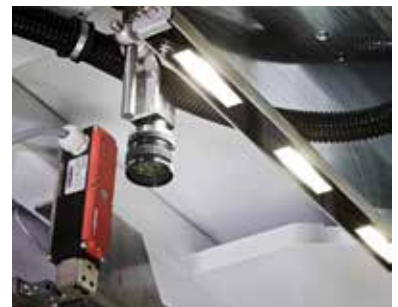
Extendable with automatic workpiece position detection by industrial imaging system
