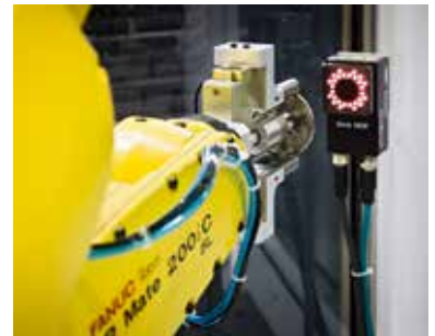
Labelling and data matrix code recognition
